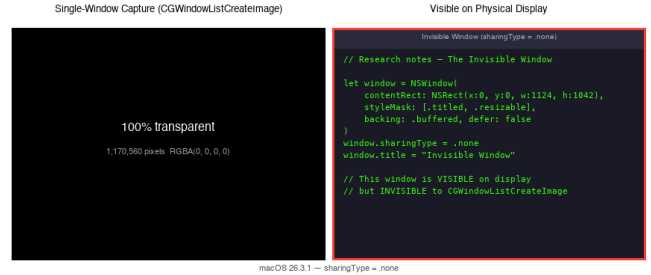
Fig. 3. macOS 26.3.1 capture comparison. Left: CGWindowListCreateImage returns a fully transparent image (1,170,560 pixels RGBA 0,0,0,0). Right: the same window as visible on the physical display. The capture pipeline renders the desktop as if the window does not exist.
